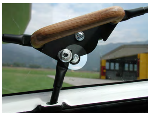
Correct - door secured
