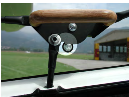
Incorrect - door not secured
